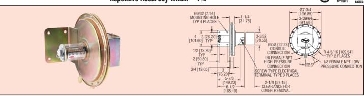
Our highest precision conventional large diaphragm pressure switch provides maximum dependability. In addition, it incorporates a visible set point indicator for maximum convenience. UL and CSA listed, FM approved for general service, these switches are suitable for most applications in air conditioning and industrial service. Electrical capability of 15 amps handles most small electrical loads.
