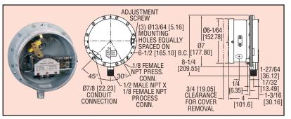
**Large diaphragm sensitivity** and time proven dependable design are combined in model PG differential pressure switches. Visible dial reduces "start up" time and helps prevent calibration errors. External adjustment allows set point change without removal of cover. Unit is listed by UL, FM and CSA.
