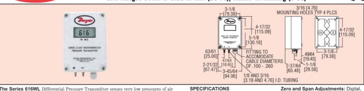
The Series 616WL Differential Pressure Transmitter senses very low pressures of air and non-combustible, compatible gases and sends a standard 4-20 mA output signal. All models, including those featuring the 3 digit LCD digital read-out, are factory calibrated to specific ranges as listed in the chart below.
