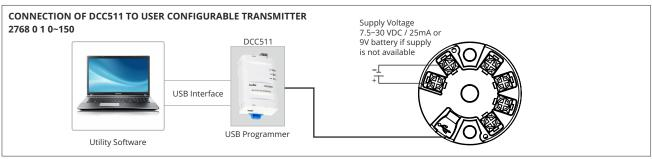
PC configurator software utility is available for calibrating/configuring transmitter using PC. DCC511 USB programmer is the hardware interface between SCC671 transmitter and PC.
