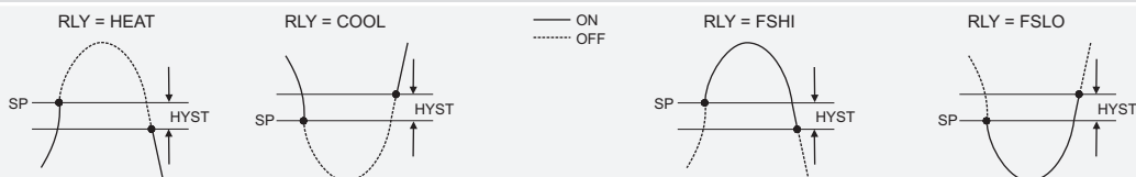
ONOFF CONTROL (Relay1, Relay2)
