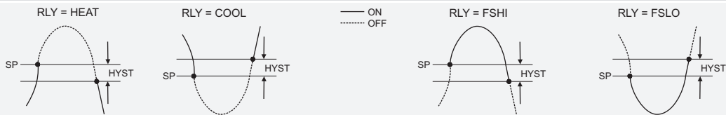
ONOFF CONTROL (Relay1, Relay2)
