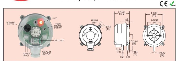
The Series BDPA Adjustable Differential Pressure Alarm with built-in audible and visual set point indication is designed for overpressure, vacuum, and differential pressure applications. The scaled adjustment knob allows changes to the switching pressure to be made without a pressure gage. The BDPA is available with settings from 0.08 in w.c. (20 Pa) to 20 in w.c. (5000 Pa). The silicone diaphragm and PA 6.6 body make the Series BDPA perfect for use with air and other noncombustible gases.
