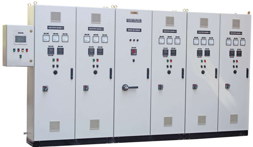
5-zone, 3-phase, SCR heating control panel Type of load : Resistive Capacity : 375kw Application : Multi zone - SS wire drawing annealing furnace
