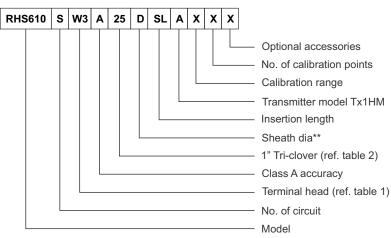
\* The deviation of RTD sensor must be added to get the measuring accuracy of the transmitter \*\* Refer table 4 for reduced tip
